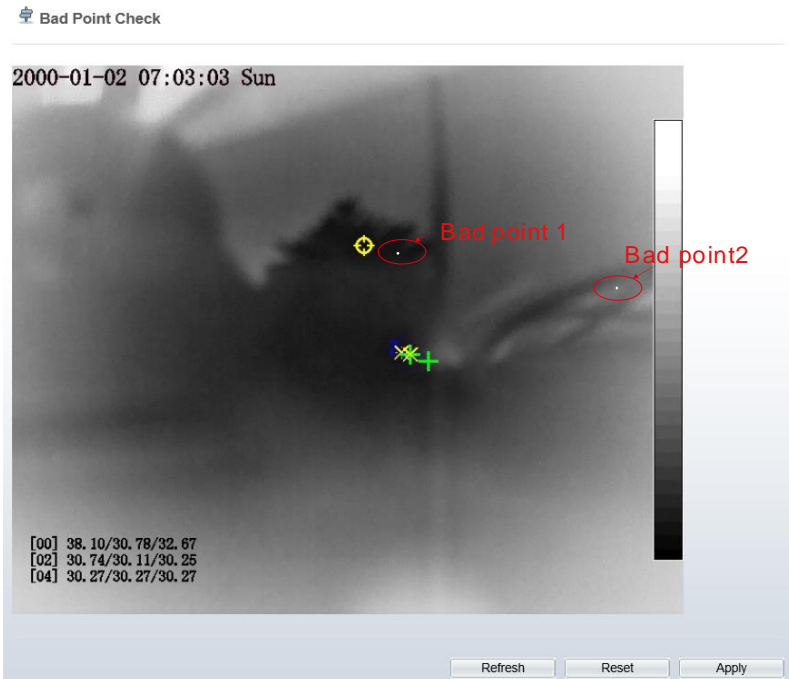
Figure 5-5 Bad Point Check
